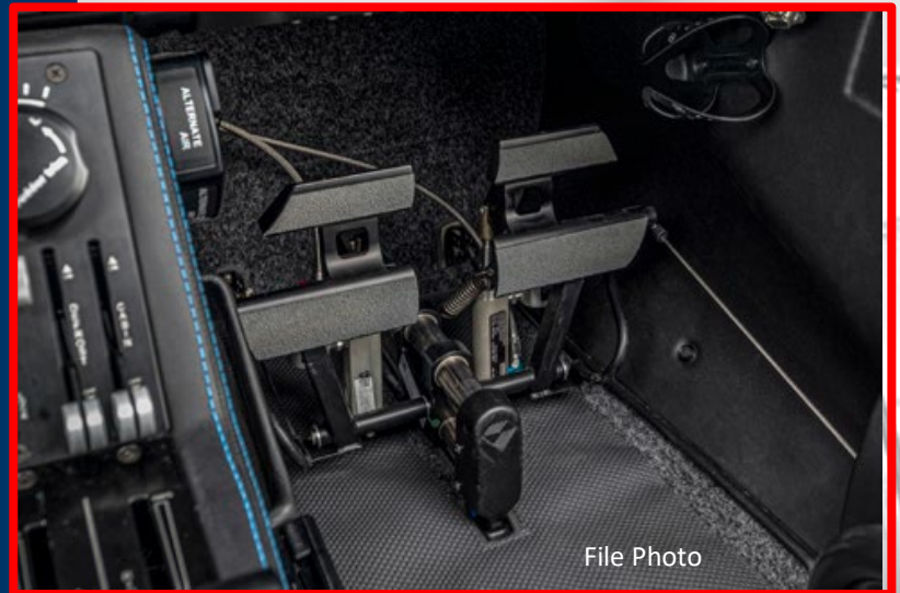
Electrically Adjustable Rudder Pedals
